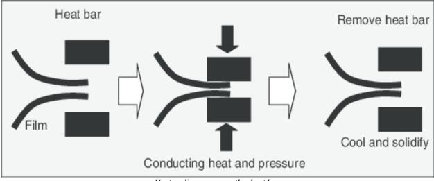
Heat sealing process with a heat bar
